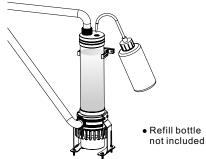
Place your PSU outside of the case and attach it to the pumps 4pin molex connector, turn on the power of PSU and make the rest of the system fills up.
