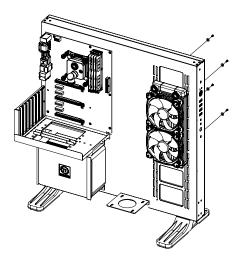
Attach the pump and reservoir into the chosen locations.
