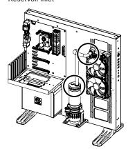
Fit the C-Pro fitting to the tube according to the order in the picture below, Install the tubes and tight the fitting caps.
