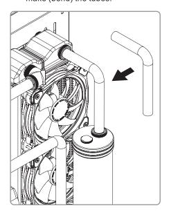
Fit the C-Pro fitting to the tube according to the order in the picture below.
